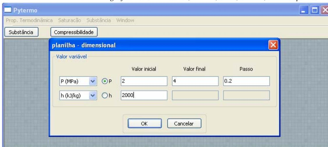
Figure 2 – A dialog for data entrance of Pytermo for dimensional thermodynamic properties determination in a range format.
